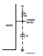
FIGURE 3. Disabling Standby Output to Eliminate C3
