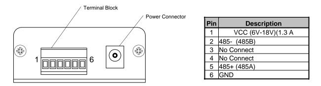
Note: Standard power is applied through the power connector. Alternative power is available via the terminal block pins.
