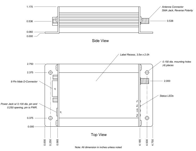
Figure 4- CL4490 Mechanical Diagram
