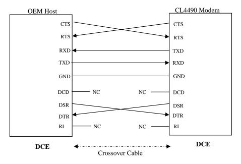
Figure 7- DCE to DCE Interface
