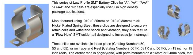
This series of Low Profile SMT Battery Clips for "A", "AA", "AAA", "AAAA" and "N" cells are especially useful in high density package applications.
