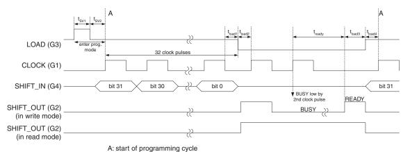
Figure 25- Serial Data Timing
