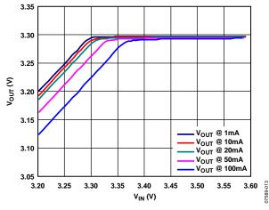
Figure 13. Output Voltage vs. Input Voltage (in Dropout), TSOT,  $V_{OUT} = 3.3 V$
