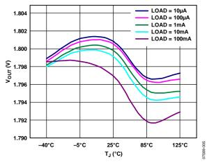
Figure 5. Output Voltage vs. Junction Temperature
