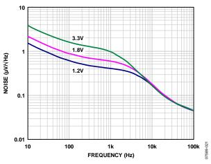
Figure 21. Output Noise Spectrum,  $V_{IN} = 5 V$ ,  $I_{LOAD} = 10 \text{ mA}$ ,  $C_{OUT} = 1 \mu F$
