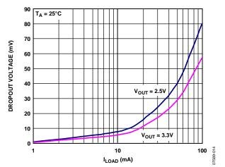
Figure 14. Dropout Voltage vs. Load Current, WLCSP,  $V_{OUT} = 2.5$  V and 3.3 V
