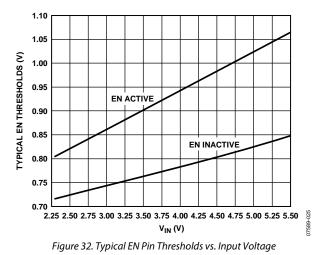
The ADP120 utilizes an internal soft start to limit the inrush current when the output is enabled. The start-up time for the 1.8 V option is approximately 120  $\mu$ s from the time the EN active threshold is crossed to when the output reaches 90% of its final value. The start-up time is somewhat dependent on the output voltage setting and increases slightly as the output voltage increases.
