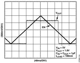
Figure 31. Typical EN Pin Operation
