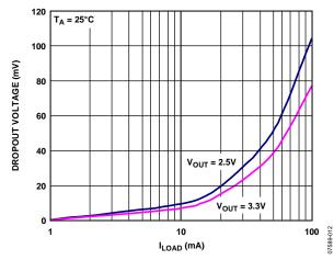
Figure 12. Dropout Voltage vs. Load Current, TSOT,  $V_{OUT} = 2.5 V$  and 3.3 V
