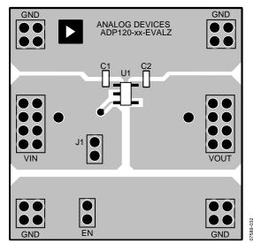
Figure 48. TSOT PCB Layout
