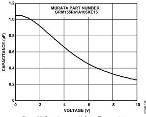
Figure 30. Capacitance vs. Voltage Characteristic
