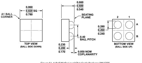
Figure 51. 4-Ball Wafer Level Chip Scale Package [WLCSP] (CB-4-2) Dimensions shown in millimeters 101507-A
