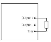
Figure 17 Output Trim Low using a Fixed resistor or Potentiometer
