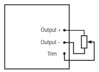
Figure 19 Variable Output Trim using a Potentiometer
