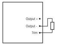
Figure 18 Output Trim High using a Fixed resistor or Potentiometer
