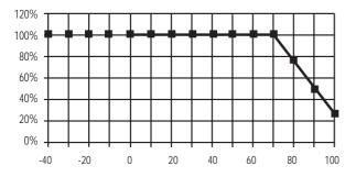
Figure 8 - Output Power versus Ambient Temperature in natural Convection
