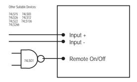
Figure 15 Implementation of Remote On/Off with TTL Devices
