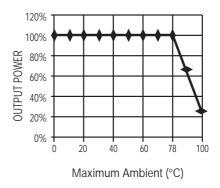
Figure 12 - Thermal Derating for 1.5m/s Forced Airflow.
