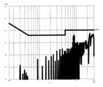
Figure 3 - EXA40-48S05 Class B Conducted Noise
