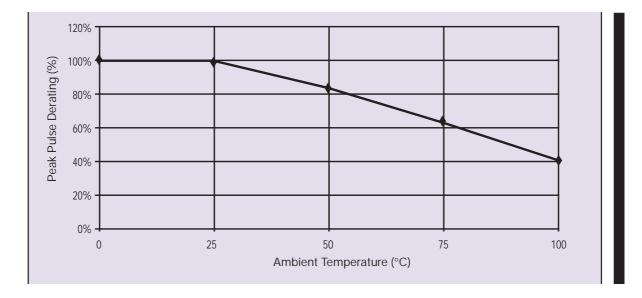
Figure A2-2 - Output TVS Peak Pulse Derating vs. Ambient Temperature
