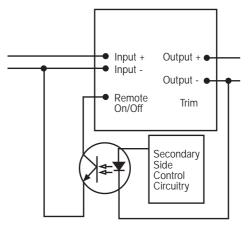
Figure 16 Secondary Side control of Remote On/Off
