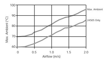
Figure 10 - Max. Ambient Temperature at full Power with Forced Airflow
