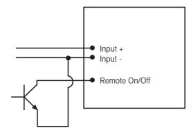
Figure 14 Implementation of Remote On/Off with a single Transistor
