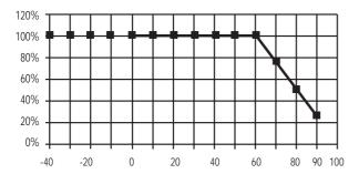
Figure 9 - Output Power versus Ambient Temperature in natural Convection for the EXA40-24S05
