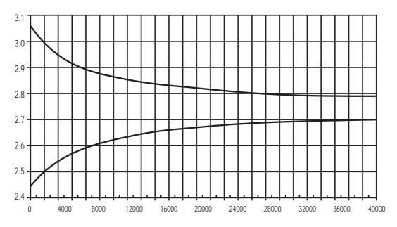
Figure A1-2 - 2.75V Output Voltage vs. Trim Resistor Value
