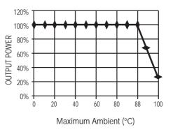
Figure 11 - Thermal Derating for 1.5m/s Forced Airflow.
