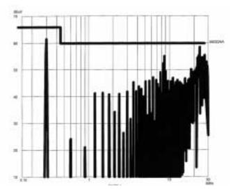
Figure 2 - EXA40-48S05 Class A Conducted Noise
