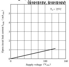
Fig. 8-b Open Circuit Leak Current vs. Supply Voltage (Typical Value)
