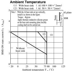
Fig. 2 RMS ON-state Current vs. Case Temperature
