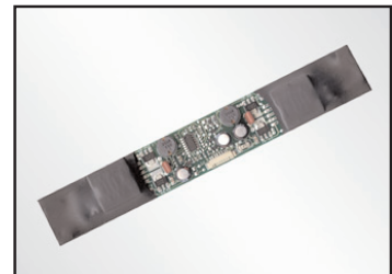
C Backlight Inverter Board (LD 2772) CAUTION: High Voltage The heat shrink tubing is used for your protection.
