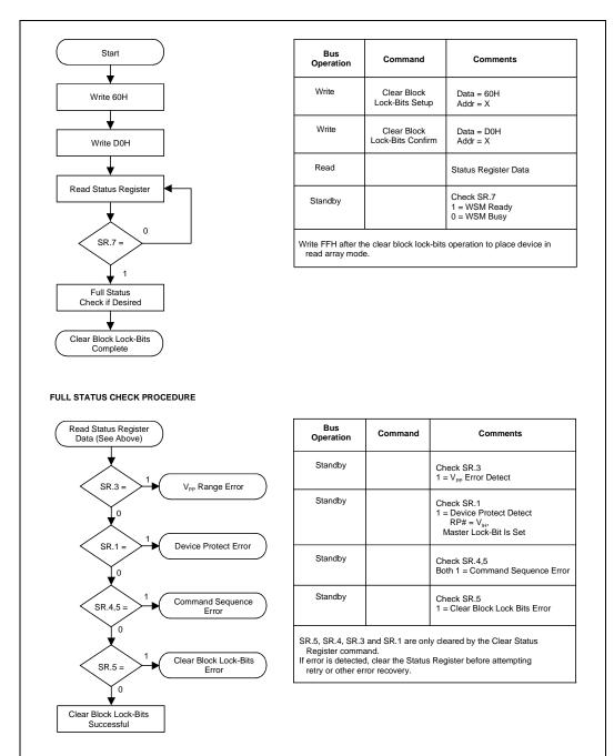
Figure 11. Clear Block Lock-Bits Flowchart
