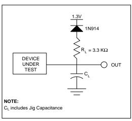
Figure 14. Transient Equivalent Testing Load Circuit
