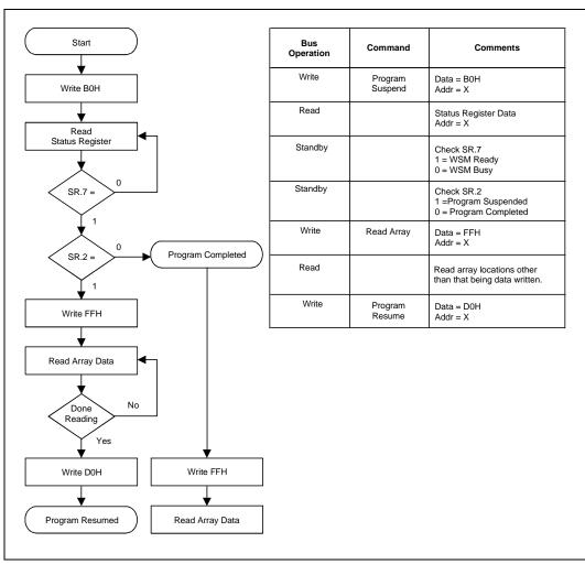
Figure 9. Program Suspend/Resume Flowchart
