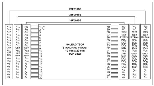
Figure 2. TSOP 40-Lead Pinout
