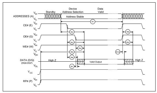
Figure 16. AC Waveform for Read Operations
