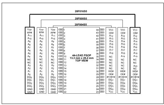
Figure 3. PSOP 44-Lead Pinout
