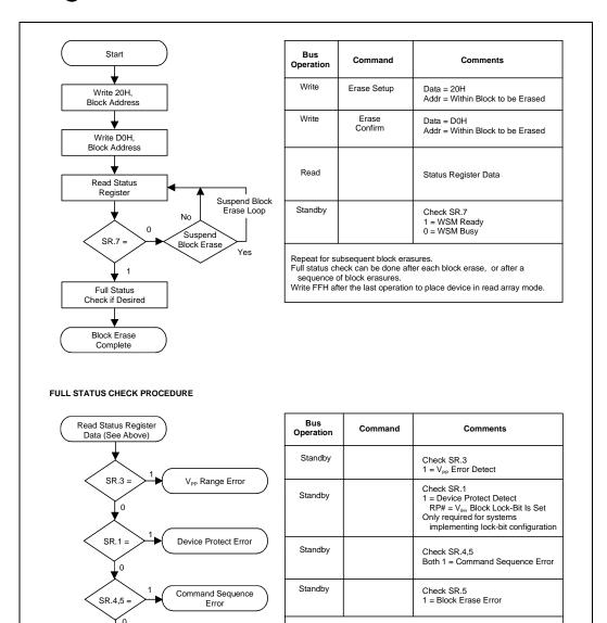
SR.5, SR.4, SR.3 and SR.1 are only cleared by the Clear Status Register command in cases where multiple blocks are erased before full status is checked.
