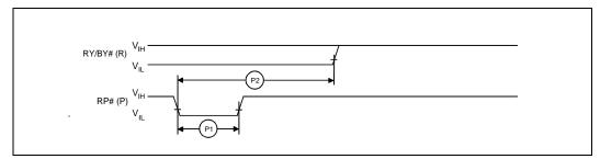
Figure 15. AC Waveform for Reset Operation
