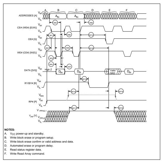
Figure 17. AC Waveform for Write Operations
