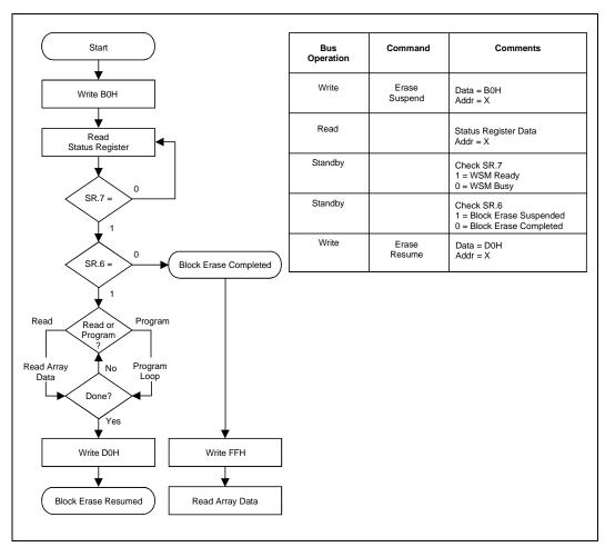
Figure 8. Block Erase Suspend/Resume Flowchart
