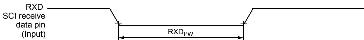
Figure 10-16 RXD Pulse Width
