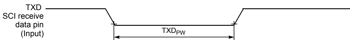
Figure 10-17 TXD Pulse Width
