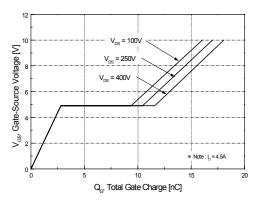
Figure 6. Gate Charge Characteristics
