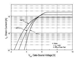
Figure 2. Transfer Characteristics
