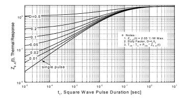
Figure 11. Transient Thermal Response Curve
