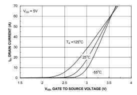
Figure 5. Transfer Characteristics.
