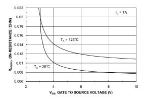
Figure 4. On-Resistance Variation with Gate-to-Source Voltage.
