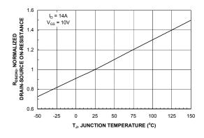
Figure 3. On-Resistance Variation withTemperature.
