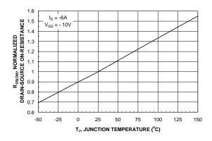
Figure 13. On-Resistance Variation with Temperature.
