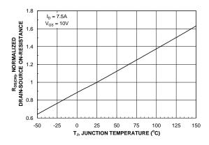
Figure 3. On-Resistance Variation with Temperature.
