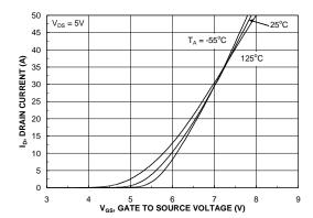
Figure 5. Transfer Characteristics.
