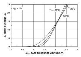
Figure 15. Transfer Characteristics.
