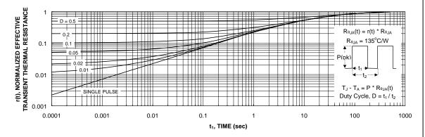
Figure 21. Transient Thermal Response Curve.
