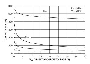
Figure 8. Capacitance Characteristics.
