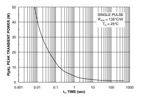
Figure 10. Single Pulse Maximum Power Dissipation.
