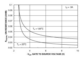
Figure 14. On-Resistance Variation with Gate-to-Source Voltage.
