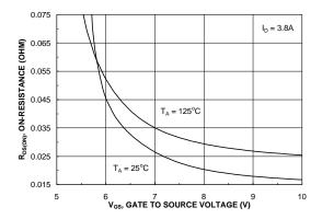
Figure 4. On-Resistance Variation with Gate-to-Source Voltage.
