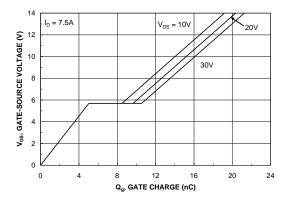
Figure 7. Gate Charge Characteristics.
