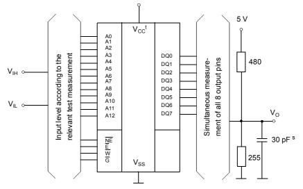
s: In measurement of  $t_{\rm dis}\text{-times}$  and  $t_{\rm en}\text{-times}$  the capacitance is 5 pF.
