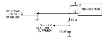
Note: Input can also be connected to  $\overline{\mathsf{DATA}}$ ; unused input pin remains unconnected. (622 Mb/s and below only.)
