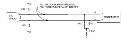
\* Locate these components as close to DATA/DATA inputs as possible.
