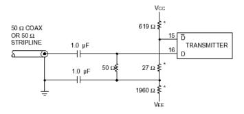
\* This network introduces a slight offset between DATA and  $\overline{\text{DATA}}$ , which turns the laser transmitter off when there is no data present at the inputs. (622 Mb/s and below only.)
