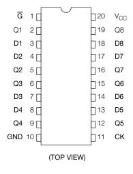
The TC74AC377 is an advanced high speed CMOS OCTAL D-TYPE FLIP-FLOP fabricated with silicon gate and double-layer metal wiring C<sup>2</sup>MOS technology.
