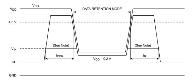
Note: When  $\overline{\text{CE}}$  is operating at the V<sub>IH</sub> level (2.2V), the standby current is given by IDDS1 during the transition of VDD from 3.6 to 2.4V.
