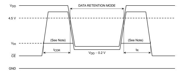
Note: When  $\overline{\text{CE}}$  is operating at the VIH level (2.2V), the standby current is given by IDDS1 during the transition of VDD from 4.5 to 2.4V.
