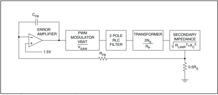
Figure 7. Current control loop block diagram.
