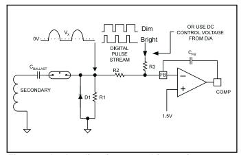
Figure 3. Analog dimming control from micro-processor.
