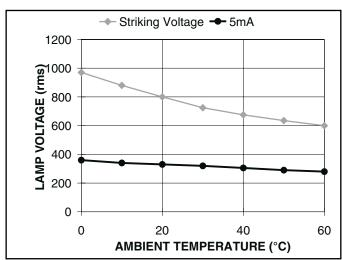
Figure 13. Temperature effects on voltage.
