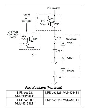
Figure 10. Optional low current shutdown circuit.
