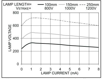
Figure 12. 3mm lamp characteristics (20 C).
