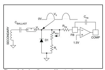
Figure 2. Analog dimmer with potentiometer.
