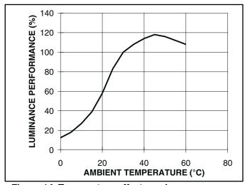
Figure 14. Temperature effects on lumens.
