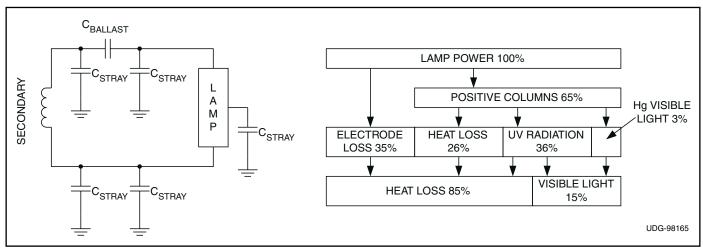
Figure 17. Lamp and stray capacitor losses.
