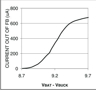
Clamp current vs. tank voltage for UCC3973.
