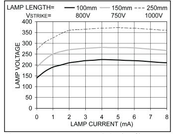
Figure 11. 6mm lamp characteristics (20 C).
