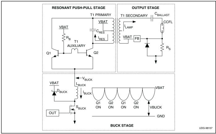
Figure 1. Push-pull, output, and buck stages.
