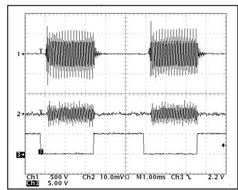
Figure 6a. LFD at 50% duty cycle.
