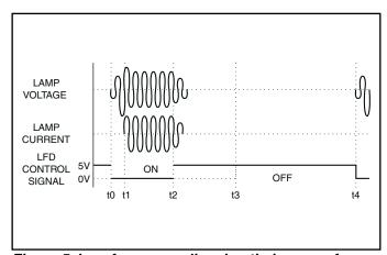
Figure 5. Low frequency dimming timing waveforms.
