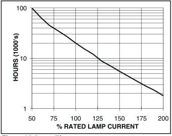
Figure 16. Lamp life versus current.
