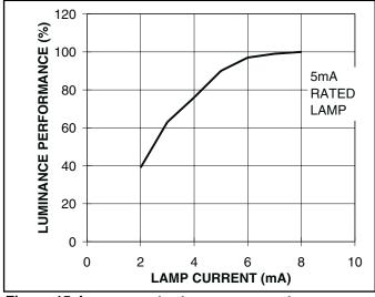
Figure 15. Lumens output versus current.
