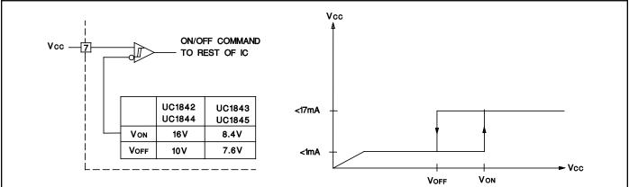
During under-voltage lock-out, the output driver is biased to sink minor amounts of current. Pin 6 should be shunted to ground with a bleeder resistor to prevent activating the power switch with extraneous leakage currents.
