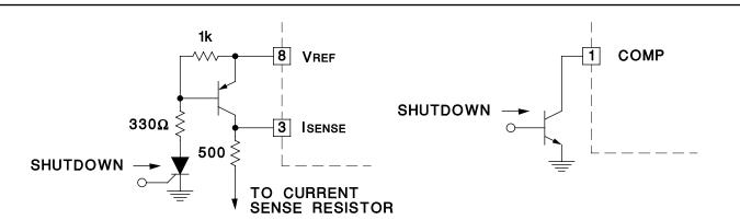
Shutdown of the UC1842 can be accomplished by two methods; either raise pin 3 above 1V or pull pin 1 below a voltage two diode drops above ground. Either method causes the output of the PWM comparator to be high (refer to block diagram). The PWM latch is reset dominant so that the output will remain low until the next
