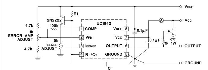
High peak currents associated with capacitive loads necessitate careful grounding techniques. Timing and bypass capacitors should be connected close to pin 5 in a
