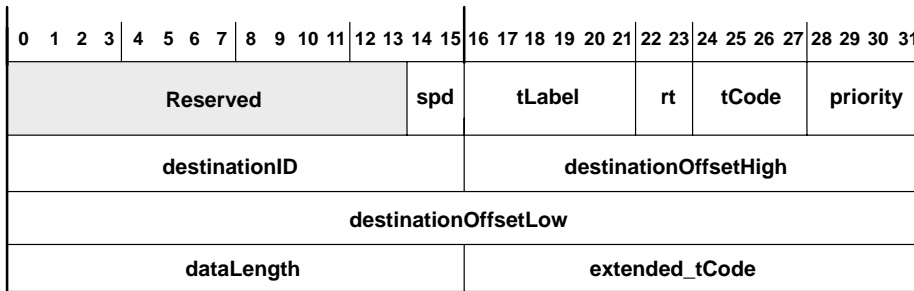
Figure 4–6. Block-Transmit Format (Read Request)
