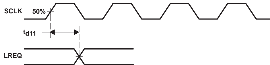
Figure 6-7. TSB12C01A Link-Request-to-Phy-Layer Waveforms
