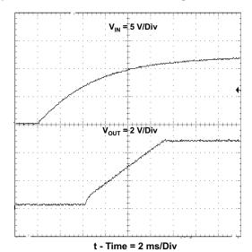
Figure 19. Startup Waveform, Vin and Vout.
