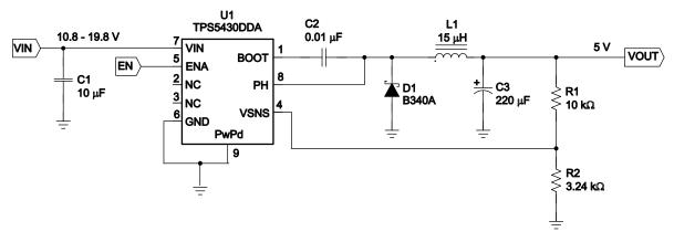
Figure 11. Application Circuit, 12-V to 5.0-V
