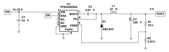
Figure 12. 12-35 V Input to 5 V Output Application Circuit
