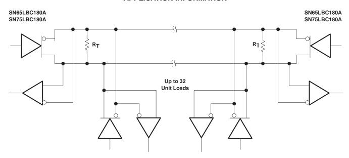
NOTE A: The line should be terminated at both ends in its characteristic impedance ( $R_T = Z_O$ ). Stub lengths off the main line should be kept as short as possible. One SN65LBC180A typically represents less than one unit load.
