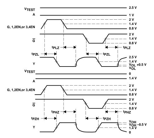
Figure 4. Enable/Disable Time Test Circuit and Waveforms
