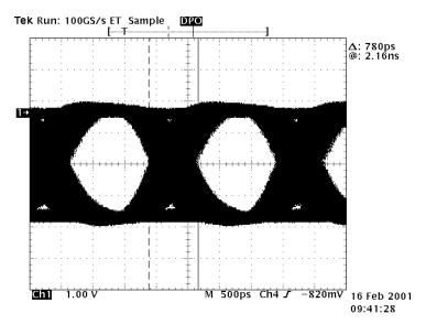
Figure 15. LV/PECL to Remote SN65LVDS32B at 500 Mbps Receiver Output (CH1)
