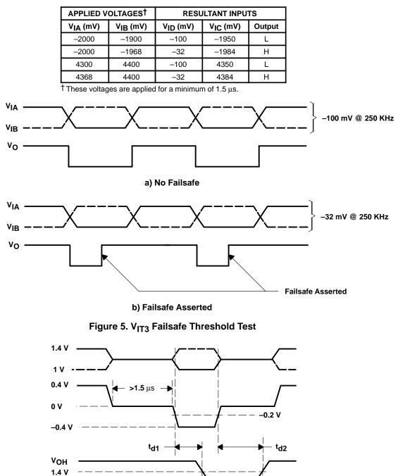
Figure 6. Waveforms for Failsafe Activate and Deactivate
