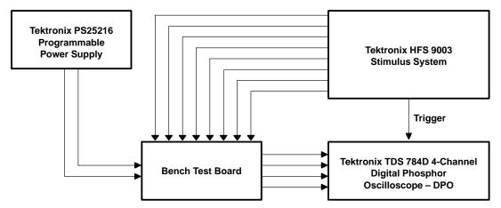
Figure 16. Equipment Setup
