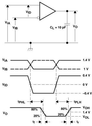
NOTE: All input pulses are supplied by a generator having the following characteristics:  $t_f$  or  $t_f \le 1$  ns, pulse repetition rate (PRR) = 50 Mpps, Pulsewidth =  $10 \pm 0.2$  ns . CL includes instrumentation and fixture capacitance within 0,06 mm of the D.U.T.
