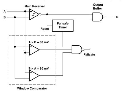
Figure 13. Receiver With Terminated Failsafe
