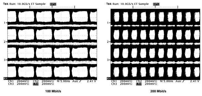
Figure 17. Typical Eye Pattern SN65LVDS32B
