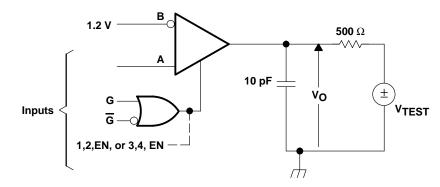
NOTE: All input pulses are supplied by a generator having the following characteristics:  $t_f$  or  $t_f \le 1$  ns, pulse repetition rate (PRR) = 0.5 Mpps, Pulsewidth = 500 ±10 ns . C<sub>L</sub> includes instrumentation and fixture capacitance within 0,06 mm of the D.U.T.
