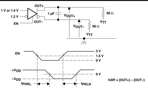
NOTE: All input pulses are supplied by a generator having the following characteristics:  $t_r$  or  $t_f \le 1$  ns, pulse-repetition rate (PRR) = 0.5 Mpps, pulse width = 500 ± 10 ns . CL includes instrumentation and fixture capacitance within 0,06 mm of the D.U.T.
