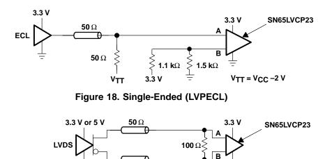
Figure 19. Low-Voltage Differential Signaling (LVDS)
