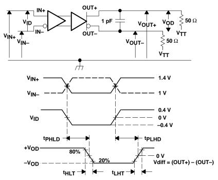
NOTE: All input pulses are supplied by a generator having the following characteristics:  $t_r$  or  $t_f \le 0.25$  ns, pulse-repetition rate (PRR) = 0.5 Mpps, pulse width = 500 ±10 ns; CL includes instrumentation and fixture capacitance within 0,06 mm of the D.U.T.
