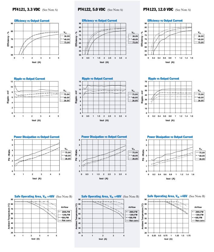
**Note A:** Characteristic data has been developed from actual products tested at 25°C. This data is considered typical data for the Converter. **Note B:** SOA curves represent the conditions at which internal components are at or below the manufacturer's maximum operating temperatures
