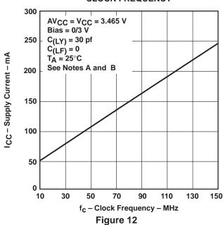
NOTES: A. C(LY) = Lumped capacitive load at Y
