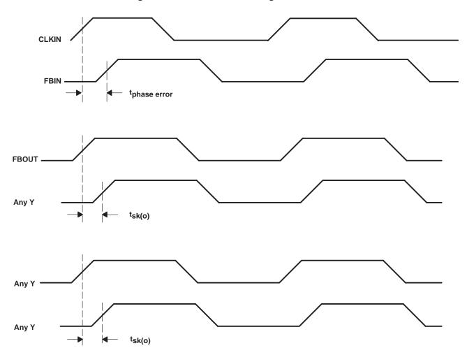
Figure 2. Phase Error and Skew Calculations
