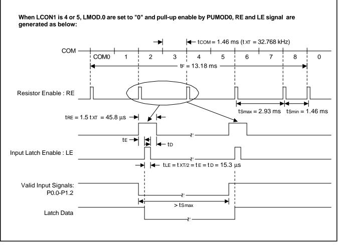
Figure 12-5. RE, LE and Inputs Signal Waveform (1/9 Duty)
