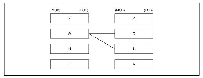
Figure 2-5. Register Pair Configuration
