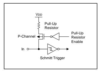
Figure 1-4. Pin Circuit Type A-3
