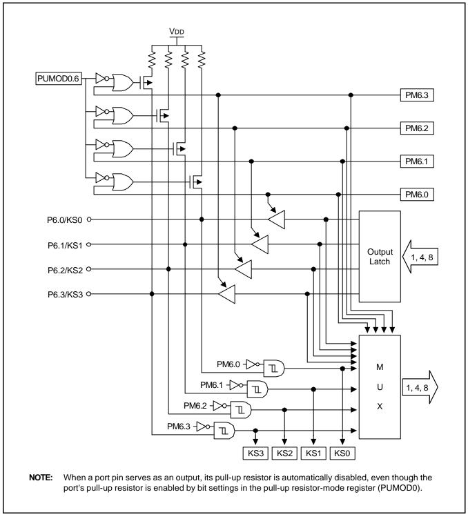
Figure 10-4. Port 6 Circuit Diagram
