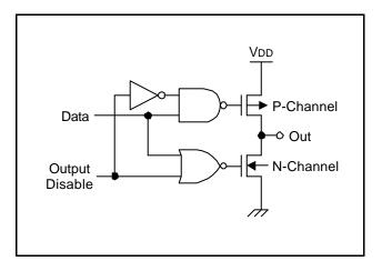
Figure 1-6. Pin Circuit Type C
