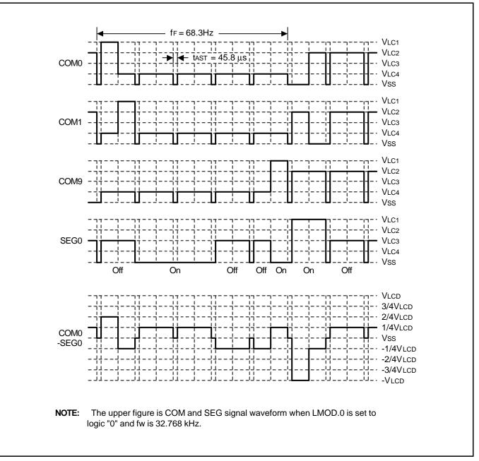
Figure 12-8. LCD Signal Waveform for 1/10 Duty and 1/4 Bias
