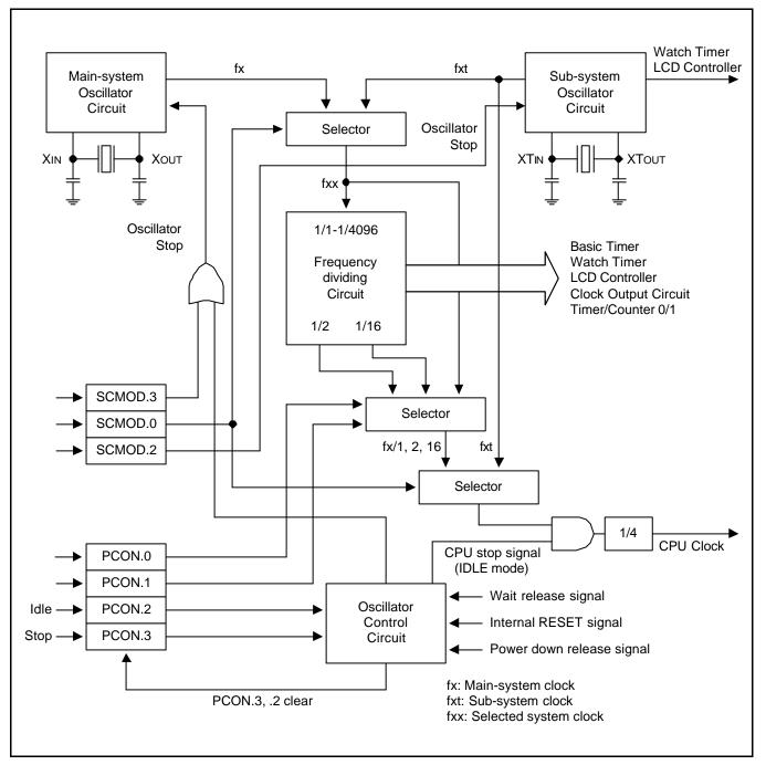
Figure 6-1. Clock Circuit Diagram
