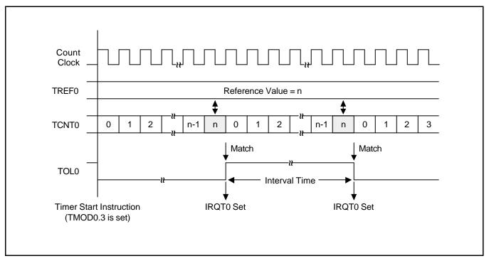
Figure 11-3. TC0 Timing Diagram
