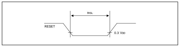
Figure 14-7. Input Timing for RESET Signal
