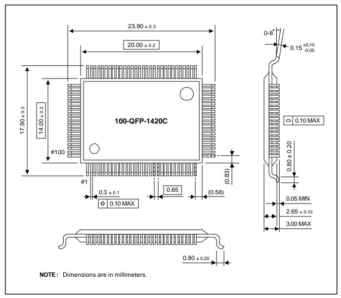
Figure 15-1. 100-QFP-1420 Package Dimensions
