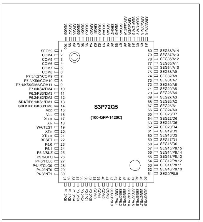
Figure 16-1. S3P72Q5 Pin Assignments (100-QFP Package)
