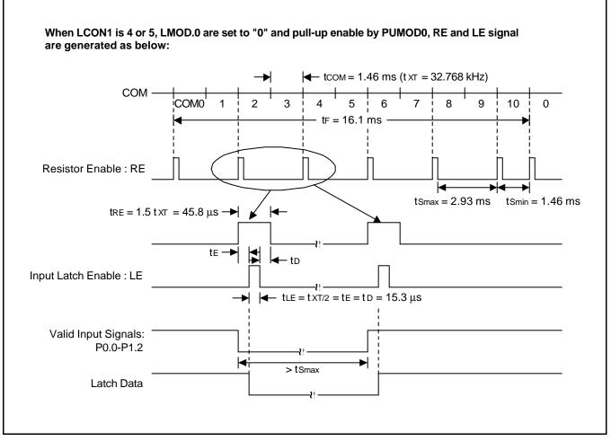
Figure 12-9. RE, LE and Inputs Signal Waveform (1/11 Duty)
