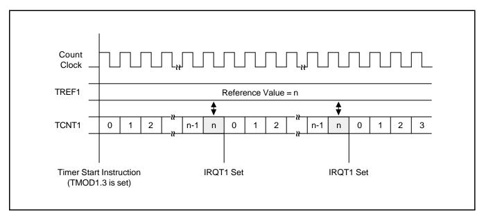
Figure 11-5. TC1 Timing Diagram
