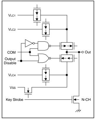
Figure 1-9. Pin Circuit Type H-4
