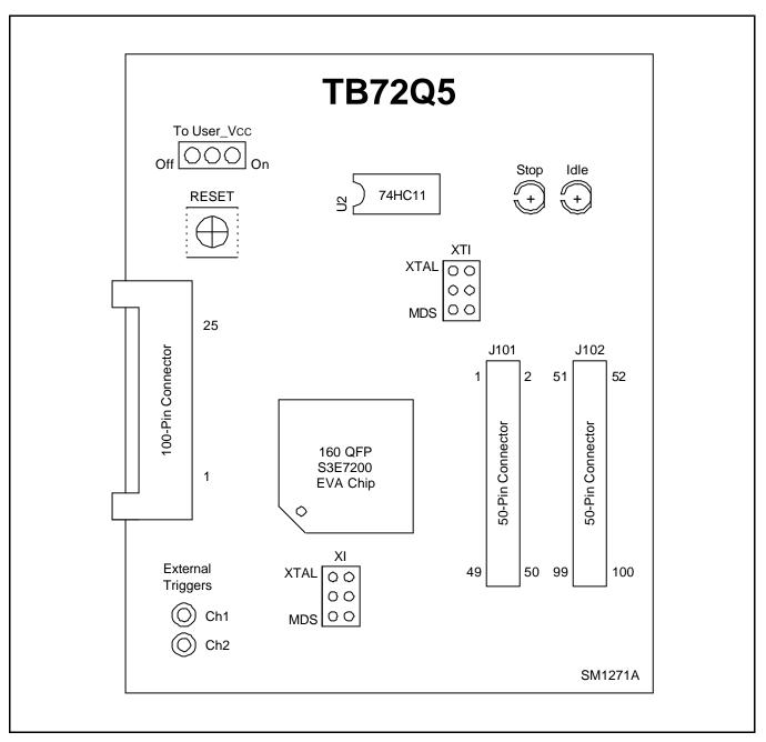
Figure 17-2. TB72Q5 Target Board Configuration
