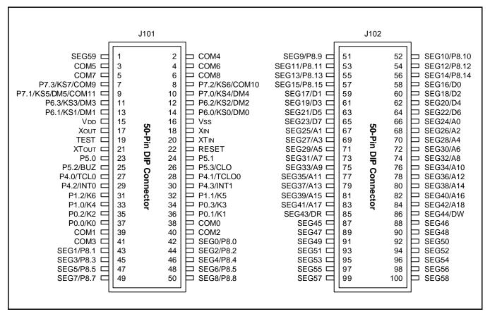
Figure 17-3. 50-Pin Connectors for TB72Q5
