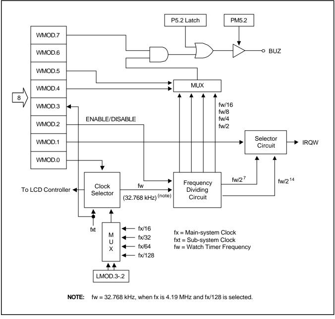
Figure 11-6. Watch Timer Circuit Diagram
