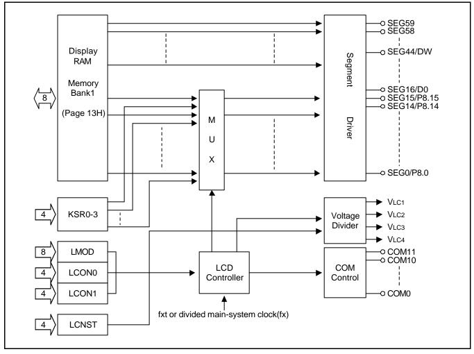
Figure 12-1. LCD Circuit Diagram
