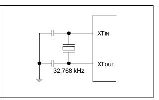
Figure 6-5. Crystal/Ceramic Oscillator
