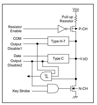
Figure 1-16. Pin Circuit Type H-12
