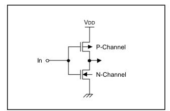
Figure 1-3. Pin Circuit Type A
