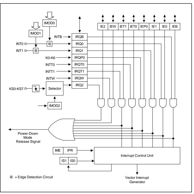
Figure 7-2. Interrupt Control Circuit Diagram
