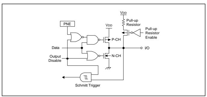
Figure 1-7. Pin Circuit Type E-2
