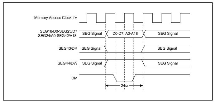
Figure 13-2. External Memory Read Cycle Timing Diagram
