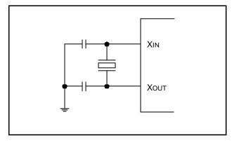
Figure 6-2. Crystal/Ceramic Oscillator
