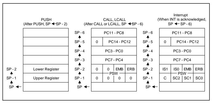
Figure 2-7. Push-Type Stack Operations
