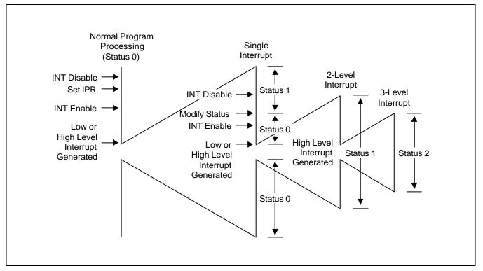
Figure 7-4. Multi-Level Interrupt Handling
