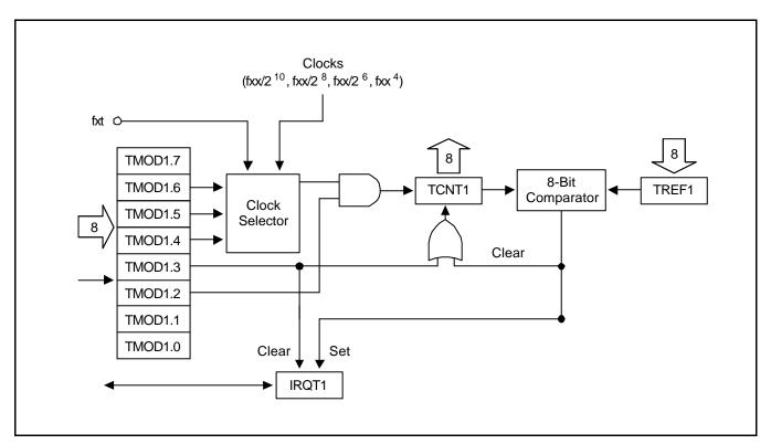
Figure 11-4. TC1 Circuit Diagram
