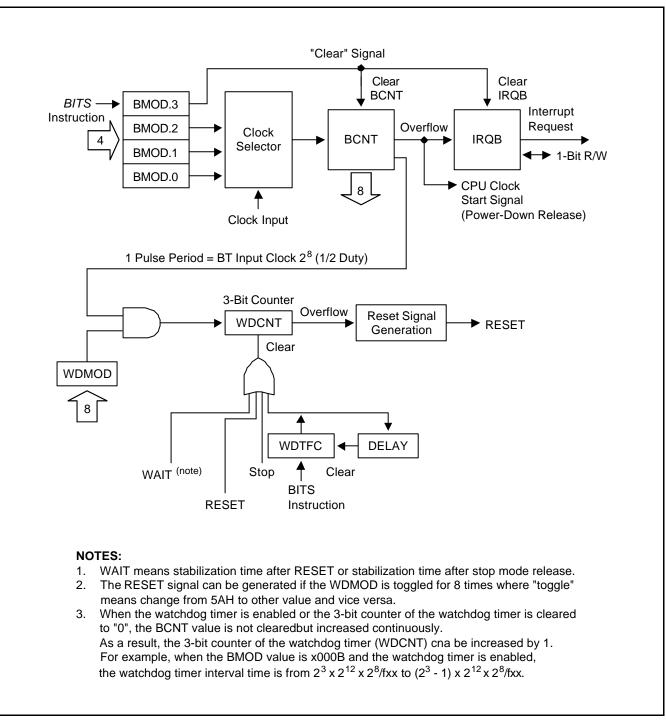
Figure 11-1. Basic Timer Circuit Diagram
