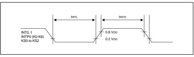
Figure 14-5. Input Timing for External Interrupts and Quasi-Interrupts
