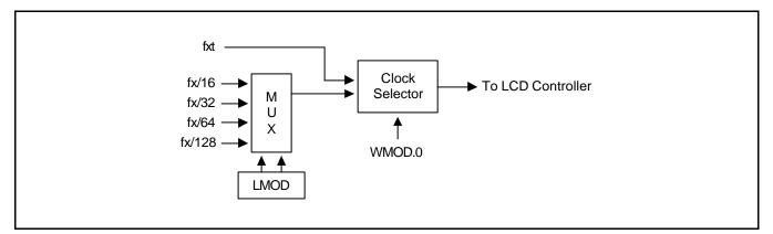
Figure 12-2. LCD Clock Circuit Diagram
