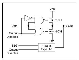
Figure 1-15. Pin Circuit Type H-11
