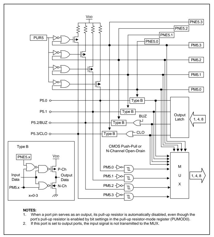
Figure 10-3. Port 5 Circuit Diagram
