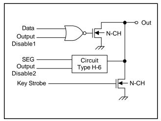
Figure 1-13. Pin Circuit Type H-9
