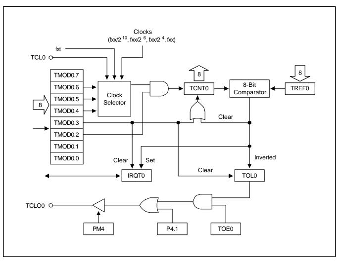
Figure 11-2. TC0 Circuit Diagram
