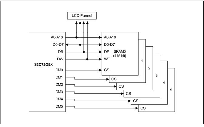
Figure 13-3. External Interface Function Diagram (S3C72Q5, SRAM, EPROM, EEPROM)
