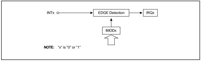
Figure 7-5. Circuit Diagram for INT0 and INT1 Pins
