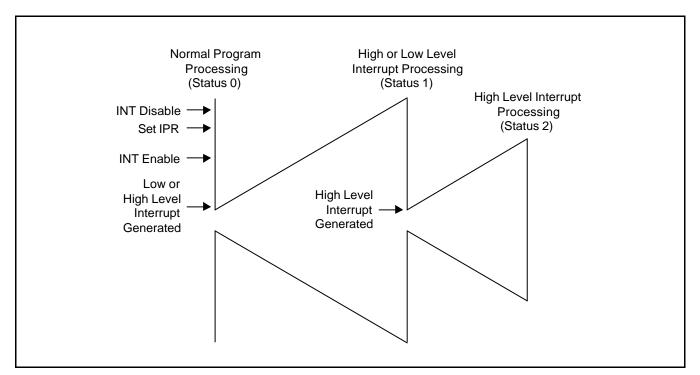
Figure 7-3. Two-Level Interrupt Handling
