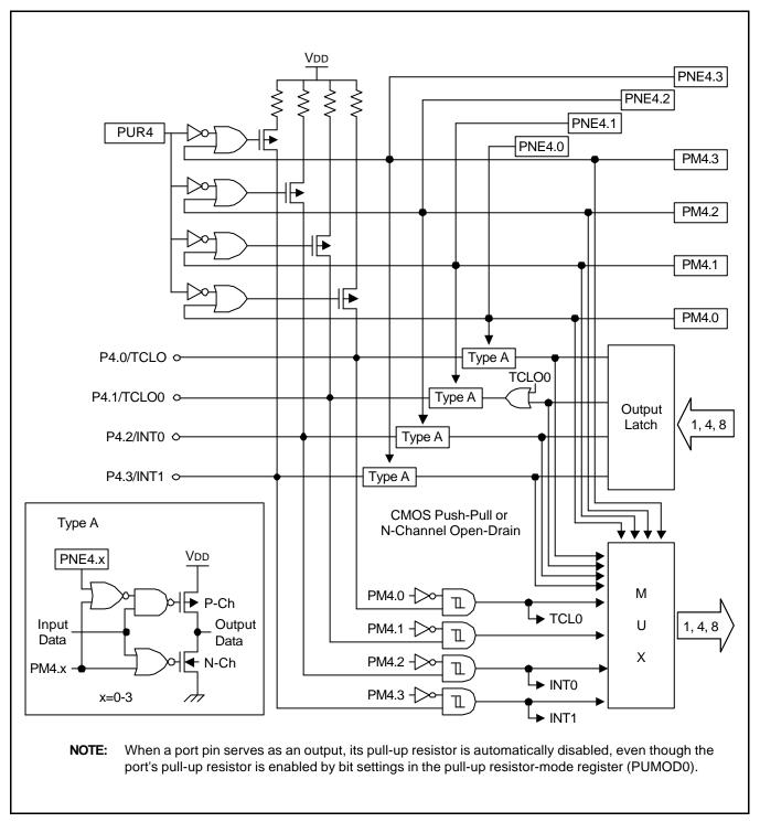
Figure 10-2. Port 4 Circuit Diagram
