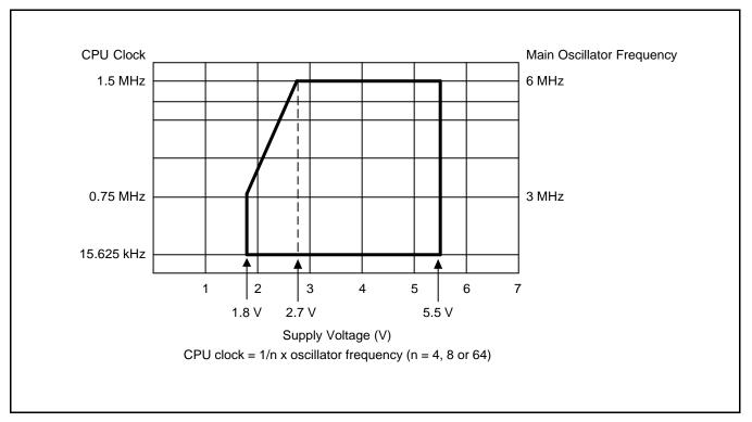
Figure 14-1. Standard Operating Voltage Range
