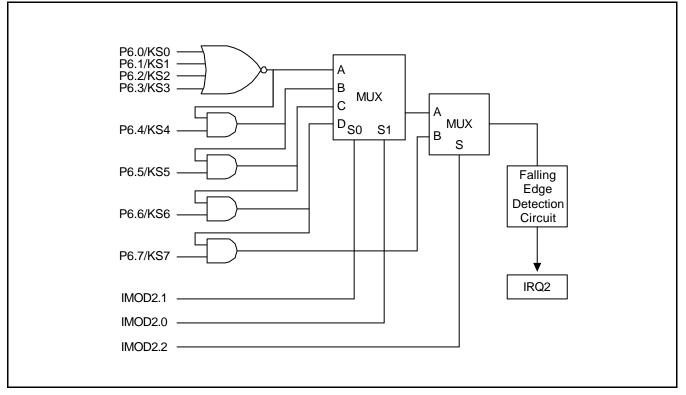
Figure 7-6. Circuit Diagram for INT2
