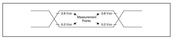
Figure 14-4. A.C. Timing Measurement Points (Except for X<sub>IN</sub> and XT<sub>IN</sub>)
