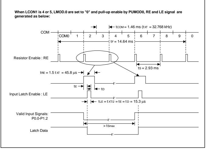
Figure 12-7. RE, LE and Inputs Signal Waveform (1/10 Duty)
