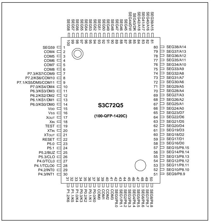
Figure 1-2. S3C72Q5 Pin Assignment Diagram
