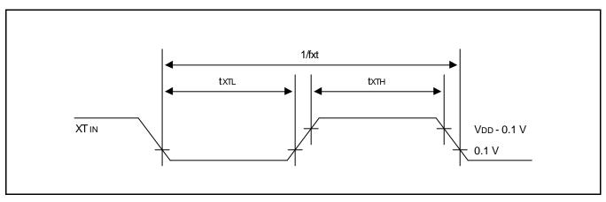
Figure 14-7. Clock Timing Measurement at  $\text{XT}_{\text{IN}}$
