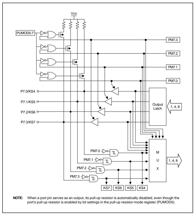
Figure 10-5. Port 7 Circuit Diagram
