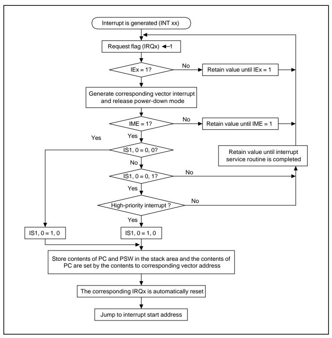
Figure 7-1. Interrupt Execution Flowchart
