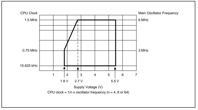
Figure 16-2. Standard Operating Voltage Range
