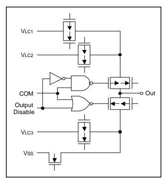
Figure 1-12. Pin Circuit Type H-7
