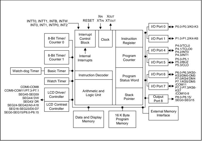
Figure 1-1. S3C72Q5/P72Q5 Specified Block Diagram
