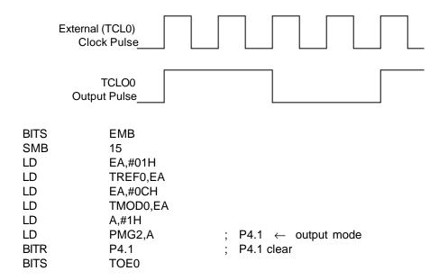
**NOTE:** The Port 4.0 must be a open-drain pin for external TC0 clock input to the TCL0 pin, when the Port 4 is set to output mode.
