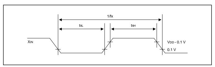
Figure 14-6. Clock Timing Measurement at  $\rm X_{IN}$
