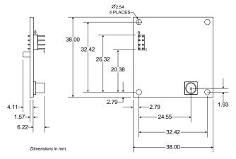
RF8001 (right angle MCX RF connector configuration)
