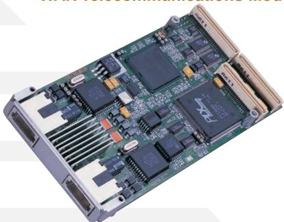
PTI's PMC370PQ Intelligent T1/E1 WAN Telecommunications Module for PMC compatible baseboards provides OEMs and integrators with two fully channelized T1/E1 interfaces for telecom and datacom applications.
