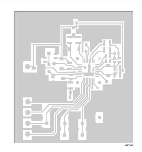
Fig.13 PCB top view for LQFP32; test circuit Figs 1 and 3.
