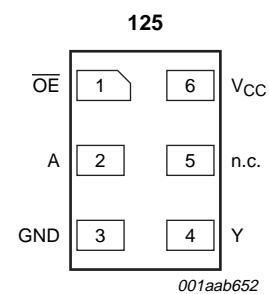
Fig.2 Pin configuration XSON6.
