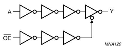
Fig.5 Logic diagram.
