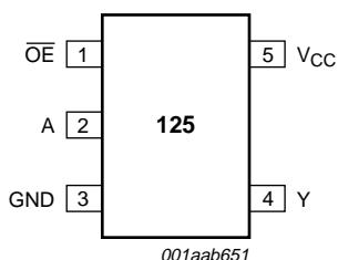
Fig.1 Pin configuration SC-88A and SC-74A.
