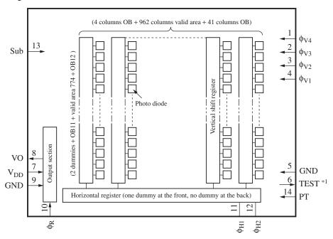
\*1 : TEST pin must be left open, because the pin outputs CCD internal bias voltage.
