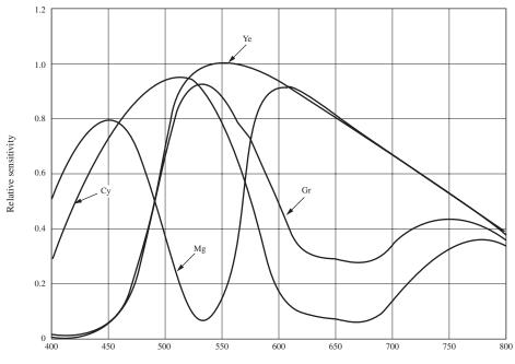
CCD color filter spectral characteristics
