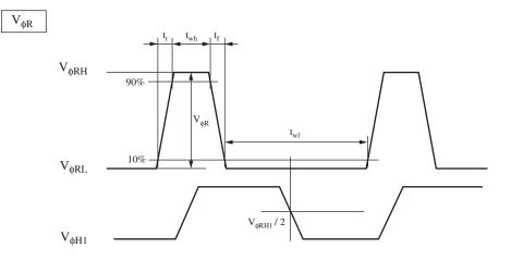
$V_{\phi RL}$  is the mean value of the waveform from the cross point of the mesial magnitude of above  $\phi_{H1}$ and  $\phi_{Rtwl}$  period to the rising point.
