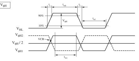
The overlap period of  $t_{wh}$  of horizontal transfer pulse  $V_{\varphi H1}$  and  $t_{wl}$  of  $V_{\varphi H2}$  and the overlap period of  $t_{wl}$ of horizontal transfer pulse  $V_{\varphi H1}$  and  $t_{wh}$  of  $V_{\varphi H2}$  are defined as  $t_{wo}$ . And VCR is the cross point voltage of the rising  $V_{\varphi H1}$  and the falling  $V_{\varphi H2}$ .
