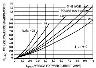
Figure 3. Average Power Dissipation
