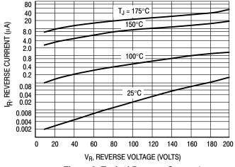
Figure 2. Typical Reverse Current\*
