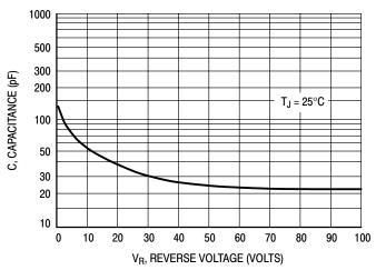
Figure 6. Typical Capacitance
