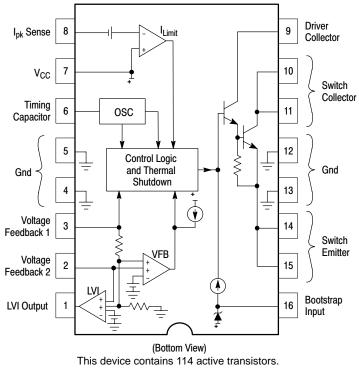
Figure 1. Representative Block Diagram
