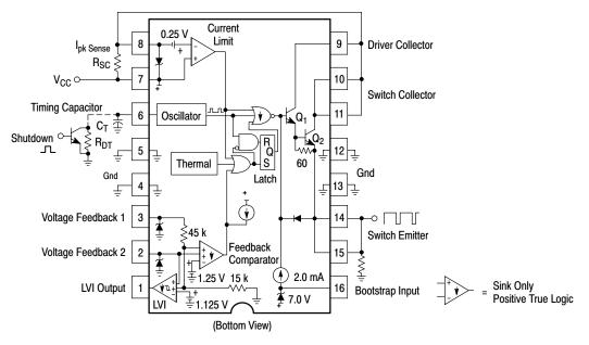
Figure 19. Representative Block Diagram
