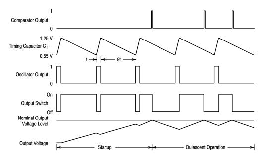
Figure 20. Typical Operating Waveforms
