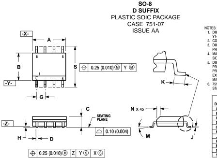
VOIES: 1. DIMENSIONING AND TOLERANCING PER ANSI Y14.5M, 1982. 2. CONTROLLING DIMENSION: MILLIMETER. 3. DIMENSION A AND B DO NOT INCLUDE MOLD DEPOTDUSION
