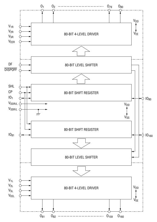
(V\_DDR/L stands for  $V_{DDR}$  and  $V_{DDL},$  and  $V_{SSR/L}$  for  $V_{SSR}$  and  $V_{SSL}.)$
