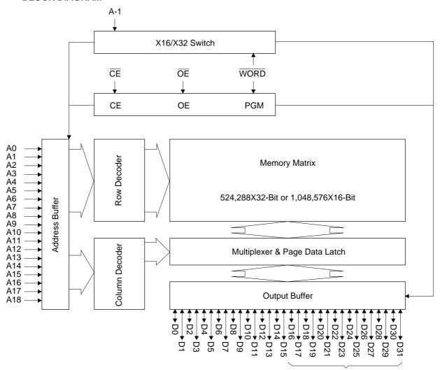
In 16-bit output mode, these pins are three-stated and pin D31 functions as the A-1 address pin.
