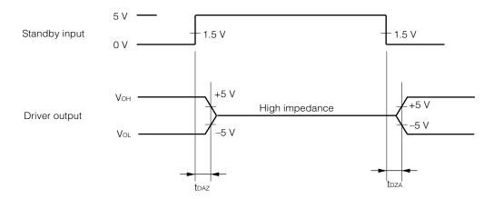
Do not perform communication within the standby output transition time  $t_{DZA}$  on power application or on releasing the standby mode.
