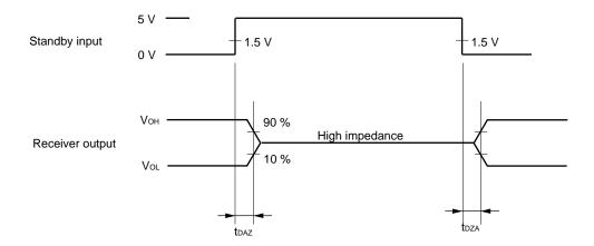
The receiver output is undefined during the standby output transition time tDZA. Do not perform communication in the standby output transition time tDZA on power application or on releasing the standby mode.
