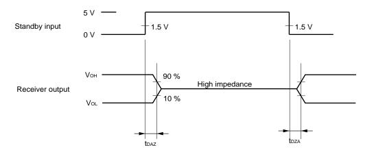
The receiver output is undefined during the standby output transition time t<sub>DZA</sub>. Do not perform communication in the standby output transition time t<sub>DZA</sub> on power application or on releasing the standby mode.
