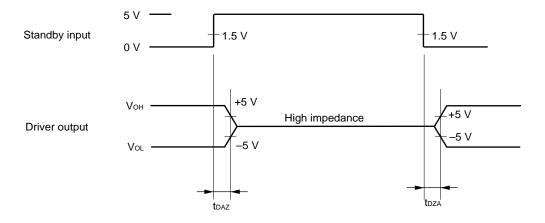
Do not perform communication within the standby output transition time t<sub>DZA</sub> on power application or on releasing the standby mode.
