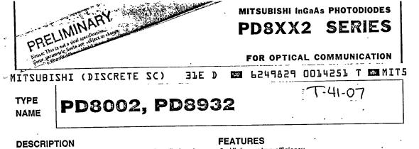
The PD8XX2 series are InGaAs avalanche photodiodes designed to operate in the wavelength range of  $1.0 \sim 1.6 \mu$ m. They provide low noise performance, low dark current, and high quantum efficiency compared with germanium avalanche photodiodes. They are well suited for wide-band and long distance fiber-optic communication systems with low transmission and low material dispersion in this wavelength range.
