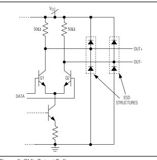
Figure 3. CML Output Buffer
