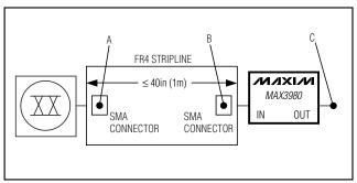
Figure 1. Test Conditions Referenced in the Electrical Characteristics Table
