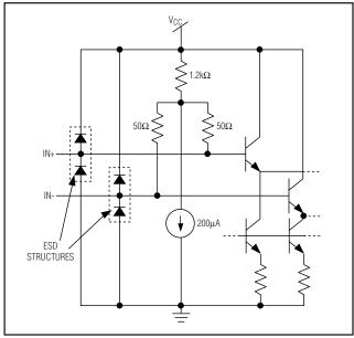
Figure 2. CML Input Buffer
