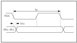
Figure 3. Definition of Clock-to-Q Delay
