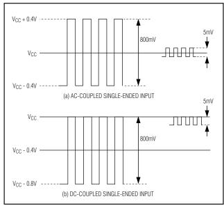
Figure 1. Definition of Input Voltage Swing
