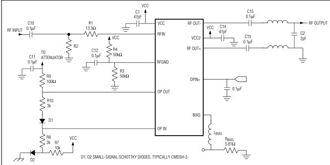
Figure 1. MAX3524 EV Kit Schematic
