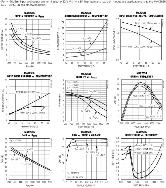
(PIN = -30dBm, input and output are terminated to  $50\Omega$ , V<sub>CC</sub> = +3V, high-gain and low-gain modes are applicable only to the MAX2656.
