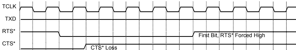
Figure 97: CTS* Loss In Synchronous Protocol: Start of Frame Waveform With CTS Lost
