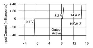
Figure 4.7 Output Current as a Function of Output Voltage
