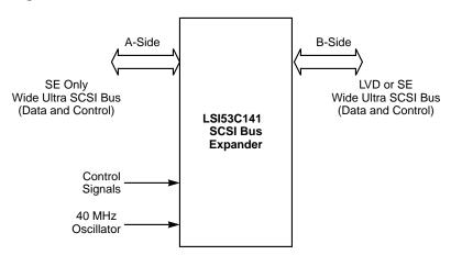
Figure 1.1 LSI53C141 SCSI Bus Device
