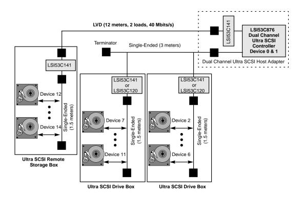
Figure 1.3 SCSI Extender or Converter Application (SE to LVD Mode of Operation)
