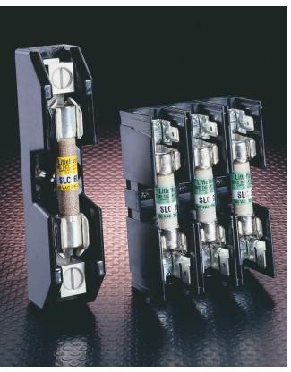
Class G fuse blocks are designed for use with 480 volt timedelay, current-limiting Class G fuses. They meet requirements for branch circuit protection.
